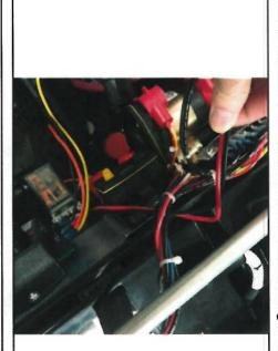
Connect the male metripack (red and black wires) from the LVI to the female metripack (red and black — wires) pigtailed with the charger blue connector.
